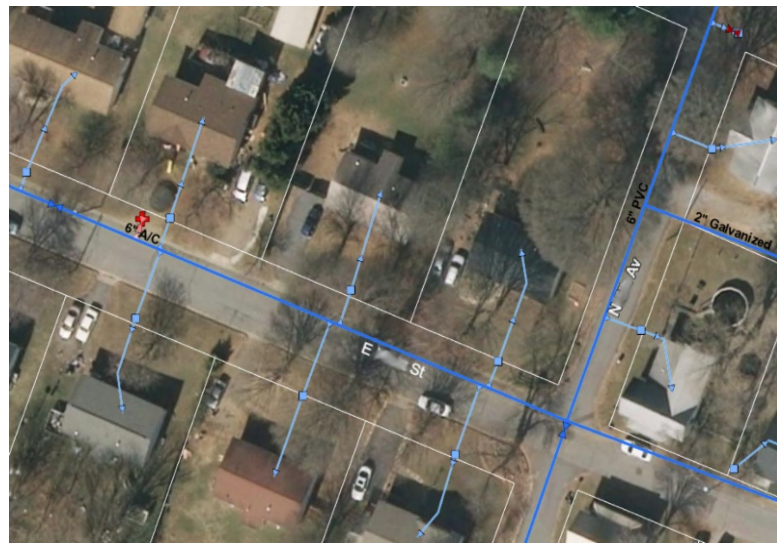
(Right) Same Area with Detail of Meters, Valves and Line Materials.
